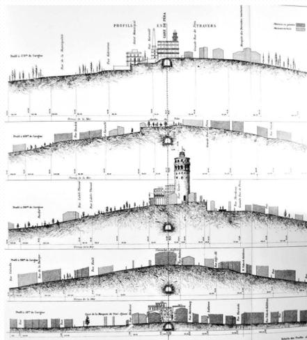
Galata Tower's location with respect to the tunnel can be seen in this figure. On the other hand the upper sectional view represents the Beyoğlu Station, the lower sectional views represent sections of the tunnel descending through sea level.
