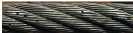
Figure 7 Fatigue-Induced Wire Breaks in Steel Wire Ropes.
