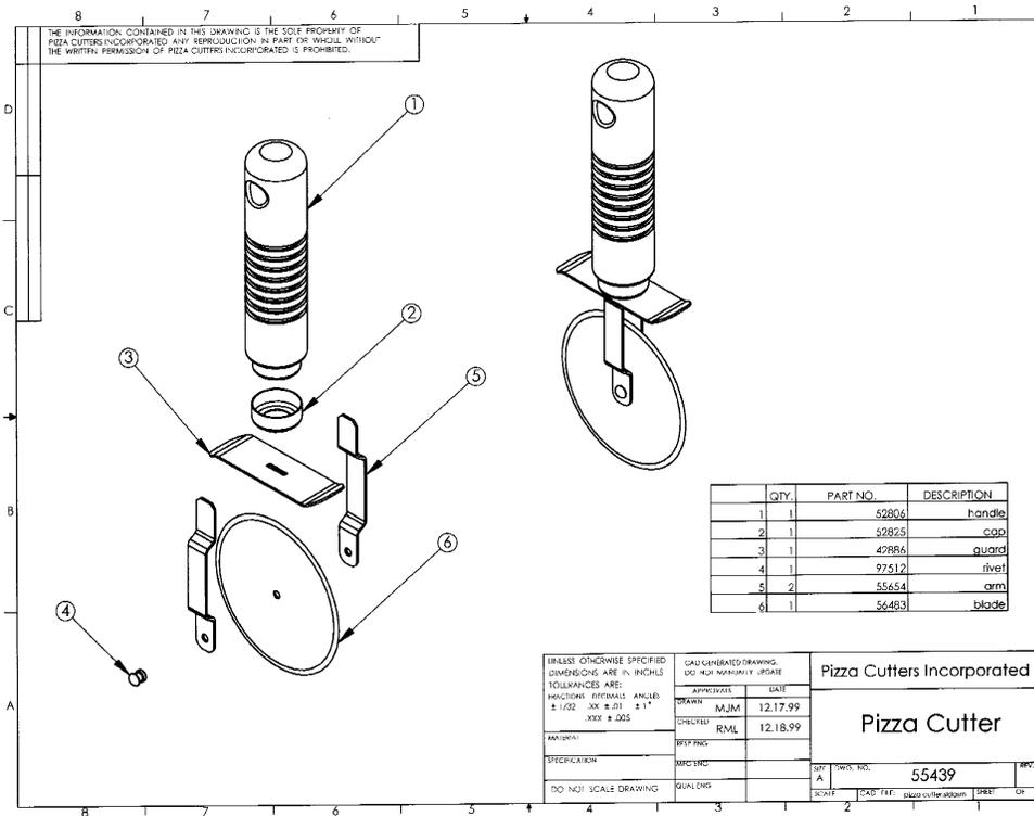
Figure 12.1 Assembly drawing of pizza cutter (from [2])
