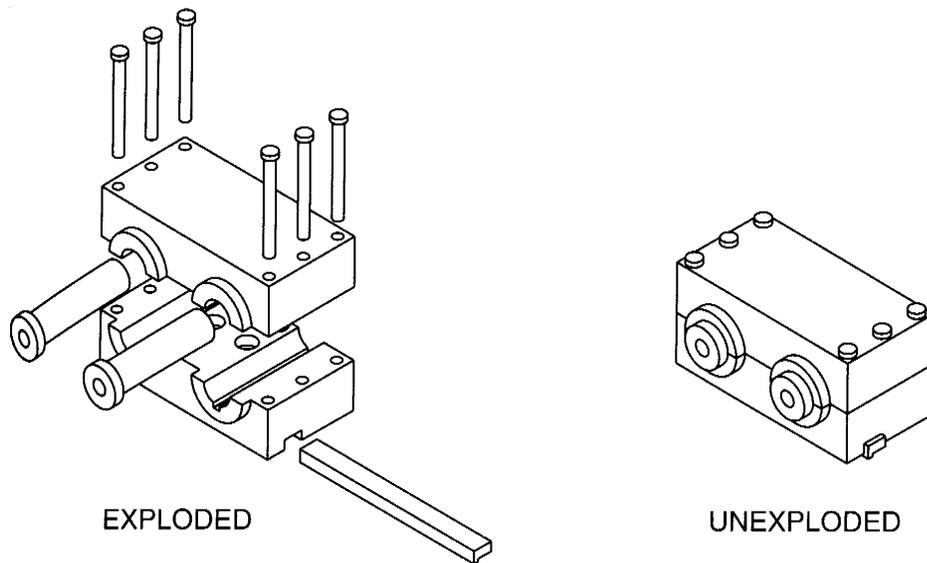
Figure 12.4. Exploded and unexploded assemblies
