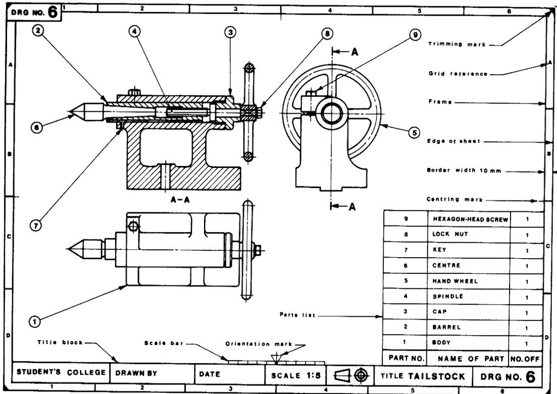
Figure 12.3. Assembly drawing with explanatory notes
