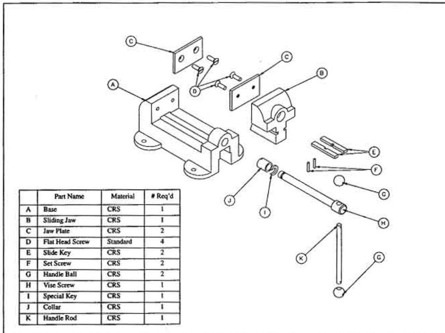
Figure 12.5. Exploded assembly drawing with bill of materials
