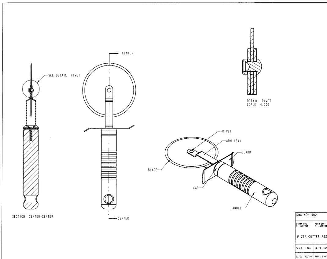
Figure 12.2 Sectional drawing of pizza cutter (from [2])
